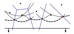
The break points move and trace out the Voronoi diagram edges
