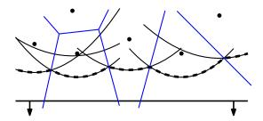
The beach line separates the known and unknown part of the Voronoi diagram, it is the minimum of the parabolas defined by sites above the sweep-line and the sweep-line itself
