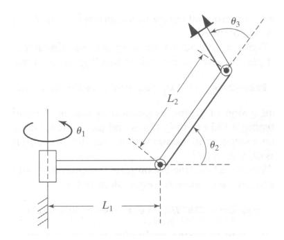
(a) (2) Assign coordinate frames to the links of the 3R arm and extract the Denavit-Hartenberg parameters of it. Then write the direct kinematics equations for the arm.
