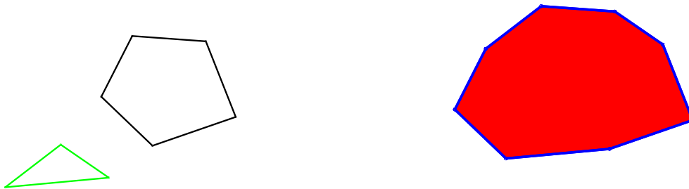
Figure 1.3: Convex input: P and Q are convex polygons with m and n vertices. The complexity of P \oplus Q is \Theta(m + n) .
