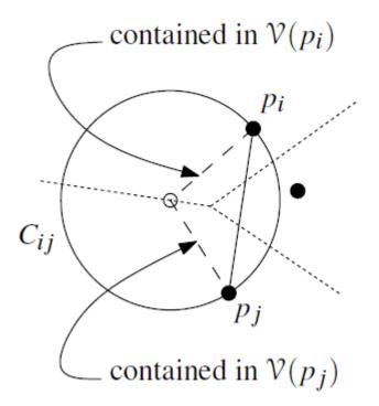
$$\begin{split} & C_{ij} \text{: an empty circle through } p_i, p_j \\ & c_{ij} \text{: the center of } C_{ij} \text{, lying on the} \\ & \text{Voronoi edge between } V(pi) \\ & \text{and } V(p_j) \\ & t_{ij} \text{: the triangle } c_{ij}, pi, pj \end{split}$$
